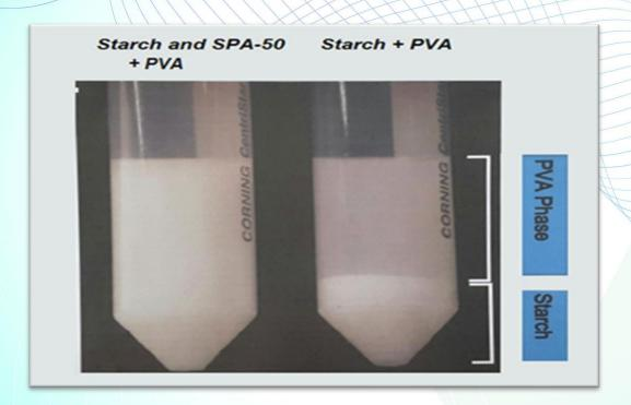
Blend of Starch and PVA are susceptible to separate in two phases. Addition of AVCO-SIZE SPA-50 eliminates this problem.
