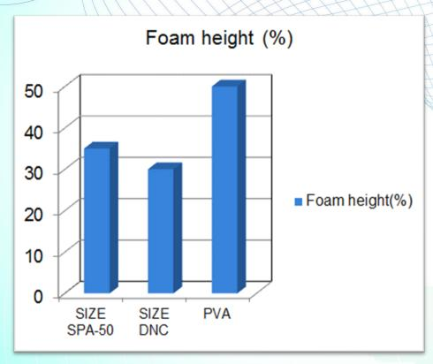
Typical result in 70/30 starch/PVA blend & AVCO-SIZE
