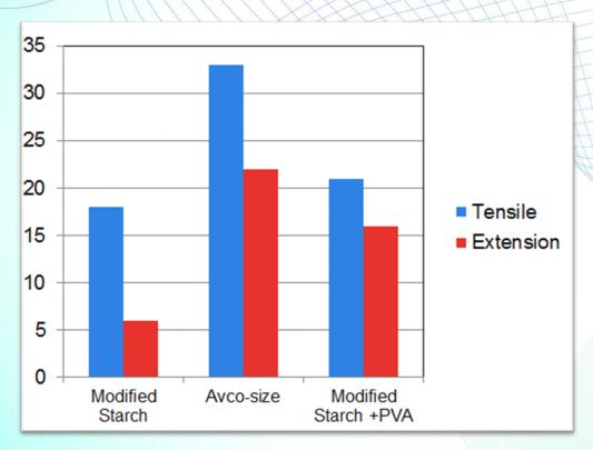
AVCO-SIZE film is stronger and tougher than modified Starch and even the blend of modified Starch and PVA
