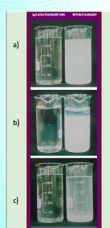
Demonstration of the efficiency of AVCO-POLYQUEST 1096 as a scale dispersing agent and as anti-precipitating agent (178 mg/l CaCO<sub>3</sub>)
